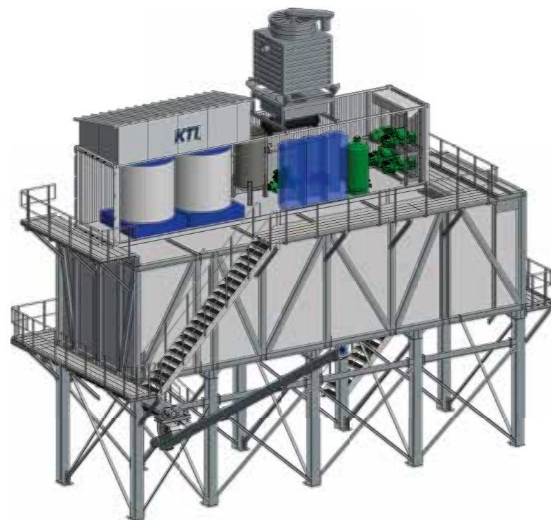
Containerized Flake Ice Plant with cooling tower on top of a Mobile Ice Storage
