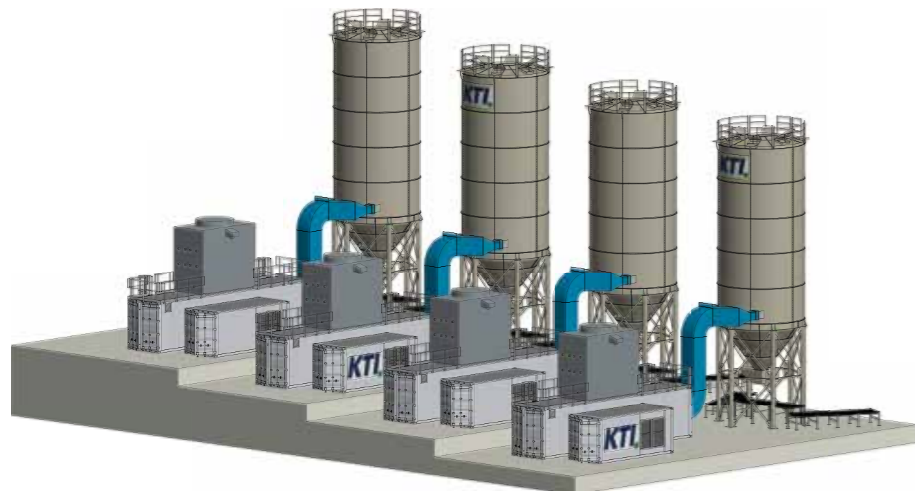
Concept layout for aggregate cooling by cold air – Live image on top
