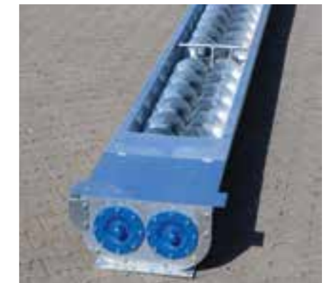
Double discharge screw conveyor
