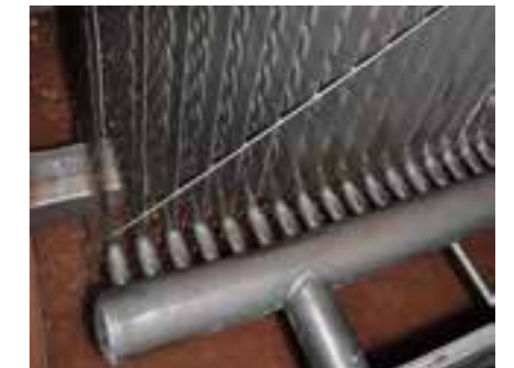
Stainless steel falling film evaporator cooling contaminated water
