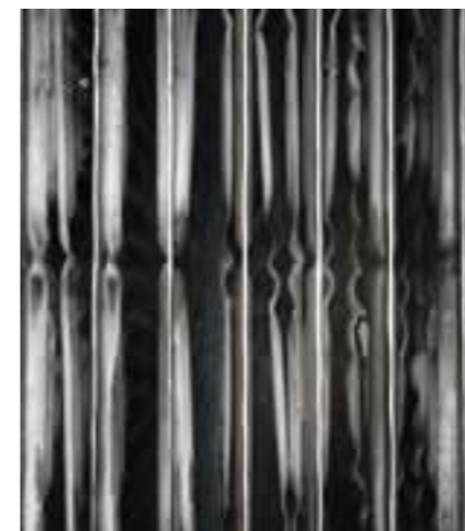
Plate Ice during harvesting by defrosting
