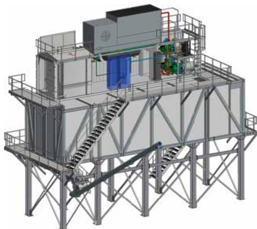
Setup with a Containerized Plate Ice Plant on top of a Mobile Ice Storage with Screw Conveyor
